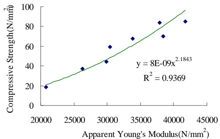
Fig.5 Relationship between the apparent Young's modulus at 200 micro strain and Compressive strength
