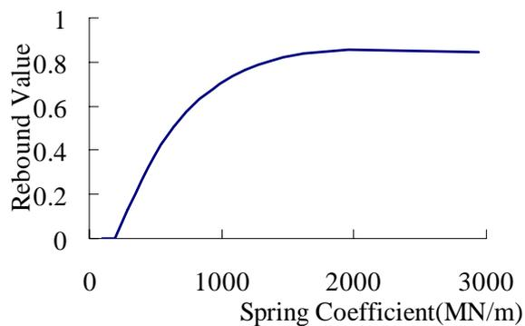
Fig.3 Relationship between spring coefficient and rebound value
