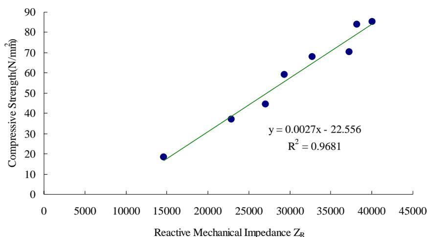
Fig.8 Relationship between compressive strength and  $Z_R$
