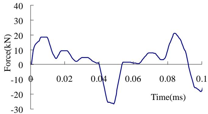
Fig.1 Calculated wave form of force on the top of plunger.
