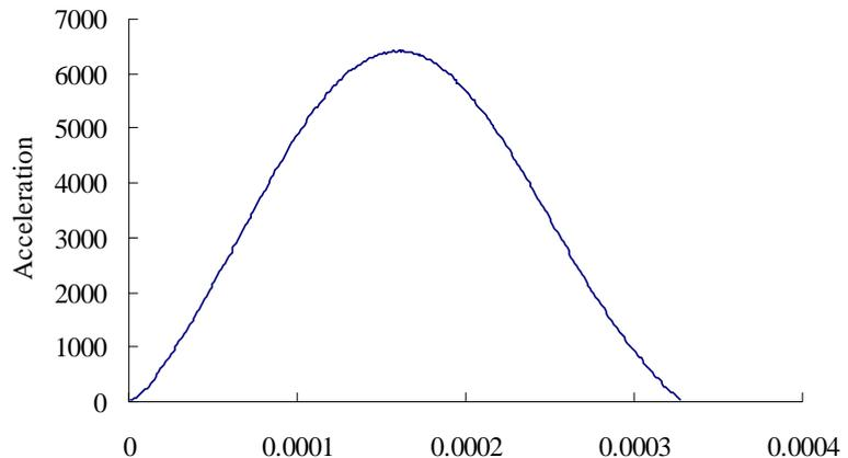
Fig.6 The typical wave form of the hammer acceleration for MC nylon
